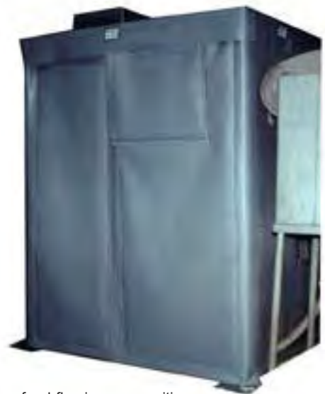
Custom feed-flap in open position (Left photo) and closed position (right photo) protects operator during loading.
